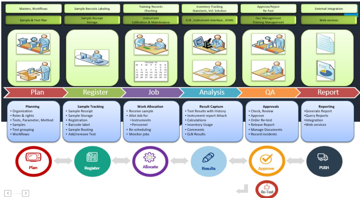
This is the overview of the sequence of process flow carried out in a typical lab. It involves: Planning, Registering, Job Allocation, Analysis or Testing, QA Verification and Approval followed by Output Report generation.
